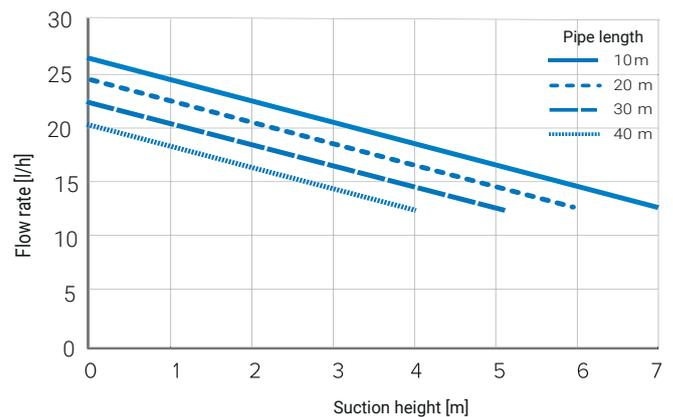
**Power loss :** for 10m horizontally, calculate a loss equivalent to 1m vertical or 0.1 bar.
