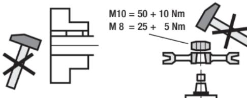
Sealing faces must not be damaged.
